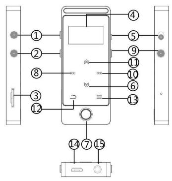
1.VOL + button 2.VOL - button 3.TF card slot 4. Display screen 5.Lock/unlock button 6. Scroll down 7.Enter/play/pause button 8. Tap for previous song 9. Power on/off button 10. Tap for next song 11.Scroll up 12.Back button 13.M button 14.Micro USB jack 15.Headphone jack
