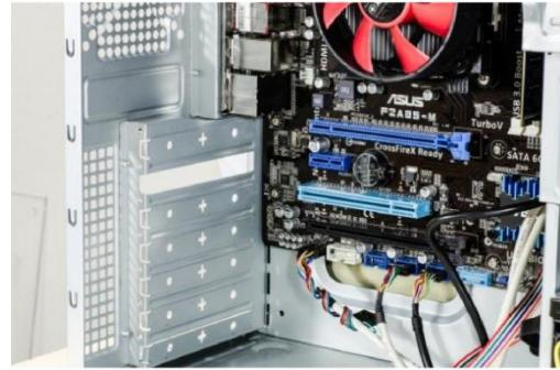
Plug the PCIe card into the slot provided. Make sure that the card sits tightly in the slot. Then use a screw to fix the card to the PC housing.
