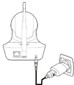
Please connect the device to the power supply,Press the device reset button.Start the device AP network.The device access point network name is:IPC\_XXXXXX.Set up wifi in the settings.
