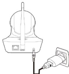
Please connect the device to the power supply and wait for more than 60 seconds. Click next to continue to add the device
