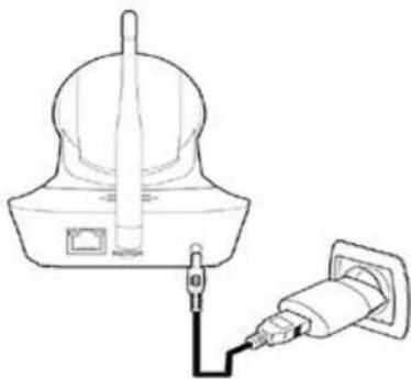
Please connect the device to power, short press the device reset button, start the device AP network, the device AP network name is IPC\_XXXXXX, connect to the device prop...
