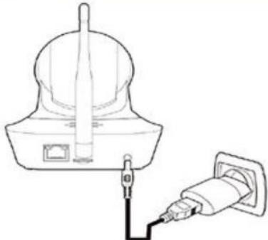
Please connect the device to power, short press the device reset button, start the device AP network, the device AP network name is IPC\_XXXXXX, connect to the device properti...
