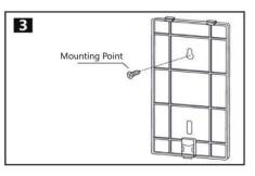
The central part of the hole is where you place the screw. Screw down with the screwdriver.
