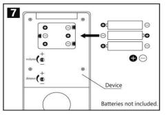
Insert the three batteries as the way shown as figure.
