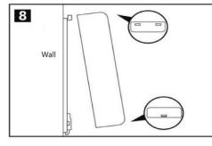
The grapnel on the back panel will buckle the hole of the main part. Press the main part towards the back panel to lock.
