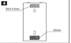
Before you install the back panel onto the wall, please paste the double-sided tape on its back.
