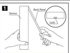
Press the button on the lower side of the back panel. Hold the back panel with one hand, then take it away from the device.
