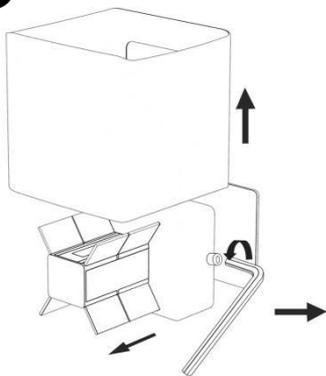
1. Remove the aluminum cover of the wall lamp. Use the included hex key to remove the base from the main body.
