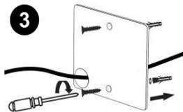
3. Drill two holes in the wall and place the included two plastic bolts into each of hole, then use the included two screws to fix the lamp base onto the wall by a screwdriver.
