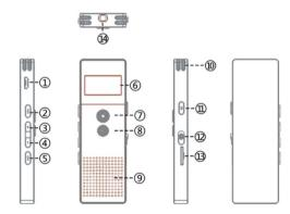
4. Volume down 11. M button 5. Previous button Switch button 6. Display screen SD card slot 7. Recording button 14. 3.5 mm Earphone Jack
