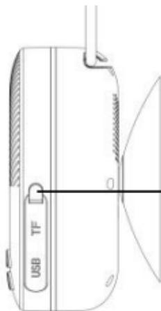
**Note:** Please tighten the Rubber Seal Cover after charging to prevent water from penetrating into the speaker.
