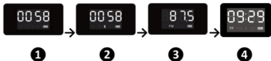
After booting up this product, this speaker will display the Time Calibration Interface ① firstly. Press **M** button to cycle through different interface, such as Bluetooth Mode ②, FM Function ③, TF Card Mode ④ (Available when TF card is inserted).
